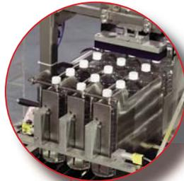
Quick clamp lane guides and numbered scales and crank adjustments enhance quick changeovers
