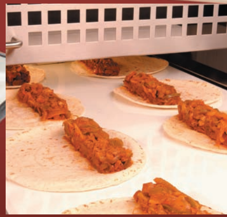
Deposits of up to 1 3/8" thick are made quickly and accurately as shown here with a tortilla application.
