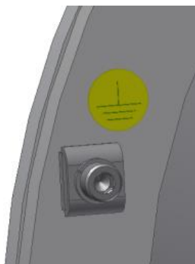
Fig. 6-4 Cutout: Example of marked central earthing connection
