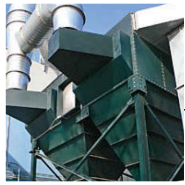
High Entry Inlet Cross flow is created through the filters. This eliminates upward “can” velocities associated with traditional hopper inlets.
