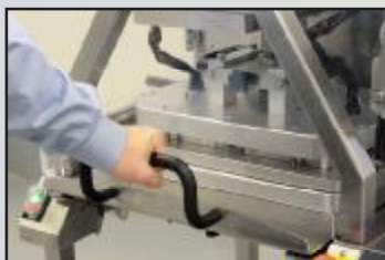
Seal head activates, flushing the product with desired gas mixture and sealing the tray.
