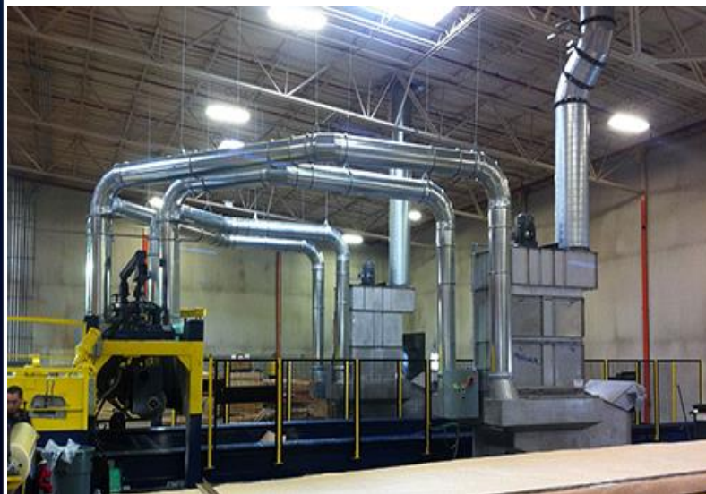
Large Polisher with pair of 12,000 cfm Stainless Collectors. Full Turnkey Installation
