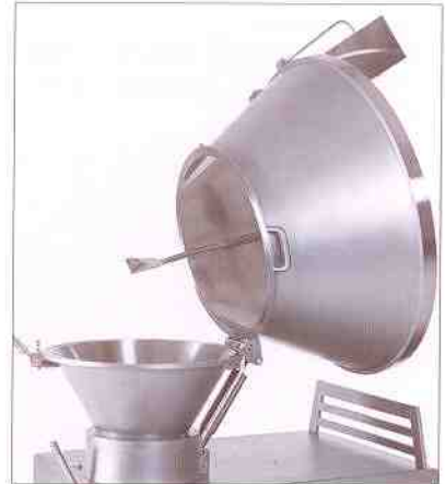
A hinge halfway up the hopper considerably facilitates cleaning when changing from one product to another.
