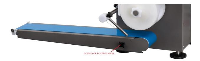
Wash the belt and platform with hot soapy water, rinse with clean water and allow to dry. Do not use strong alkaline/acid based cleaners.
