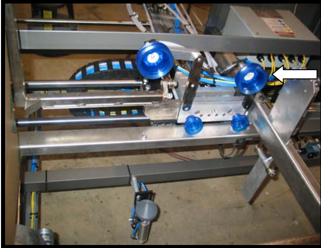
Figure 7A and 7B. Vacuum cups can be adjusted for correct placement for varying case sizes. (See set up procedures).
