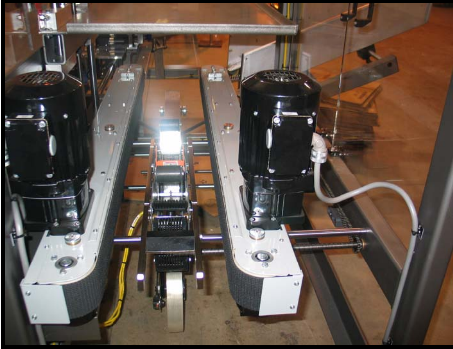
Figure 10. Side Belts and Motors.
