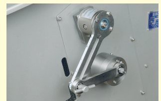
Enlarged thickness adjuster right side
