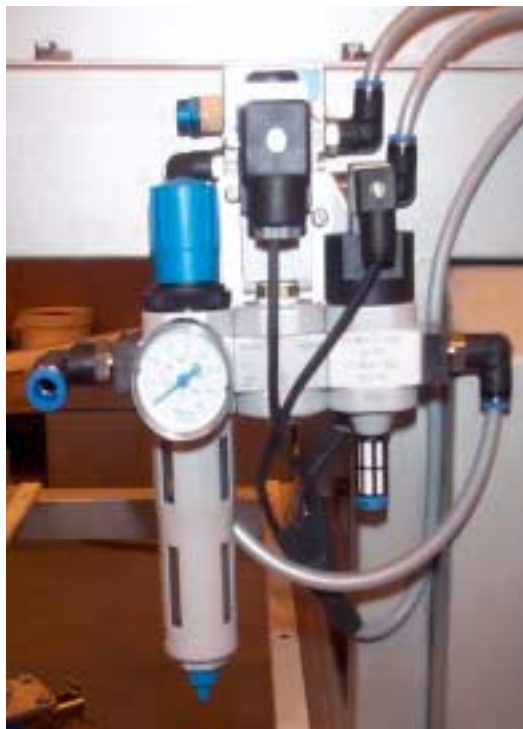
Figure 8.9 Pusher and Plough Reject
