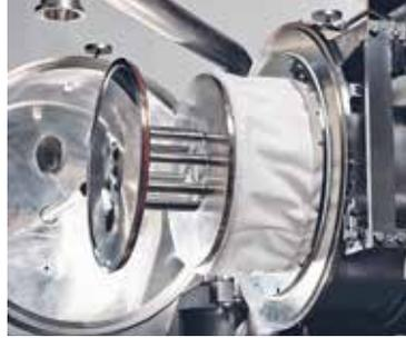
Discharge with inverted filter cloth
