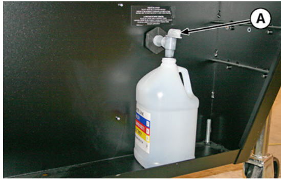
Figure 10-24 Waste ink bottle and spigot
