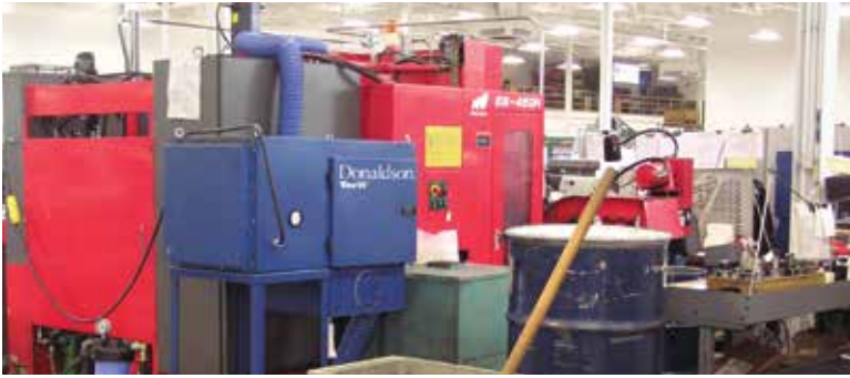
DMC on Machining 800 cfm (1,359 m 3 /h)
