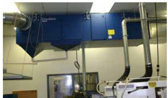
MODULAR MEDIAFILTER™ on Grinding 2,000 cfm (3,397 m 3 /h)
