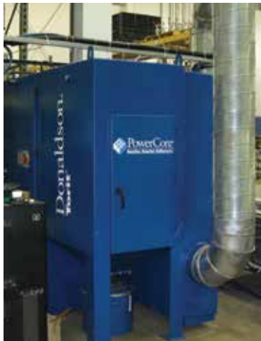
TG on Plasma Cutting 2,300 cfm (3,90 m 3 /h)
