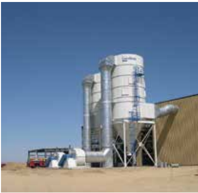
LP on Nut Dust 280,000 cfm (475,622 m 3 /h)
