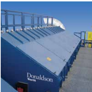
CPC - Grain Tripper Conveyor 18,700 cfm (31,765 m 3 /h)
