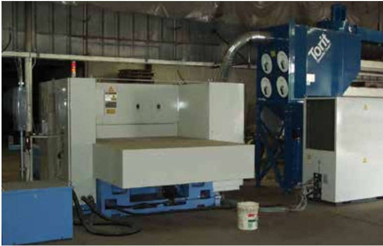
DFO on Laser Cutting 3,100 cfm (5,266 m 3 /h)
