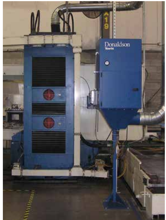
WSO - Horizontal Grinder 850 cfm (1,444 m 3 /h)
