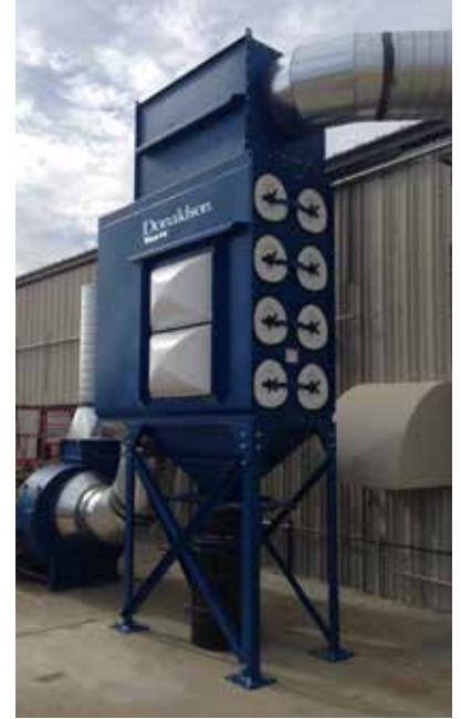
DFO on Plastics Routing 16,000 cfm (27,184 m³/h)
