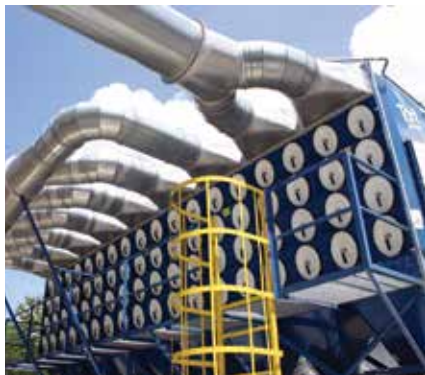
DFO on Sawdust 57,500 cfm (97,692 m 3 /h)
