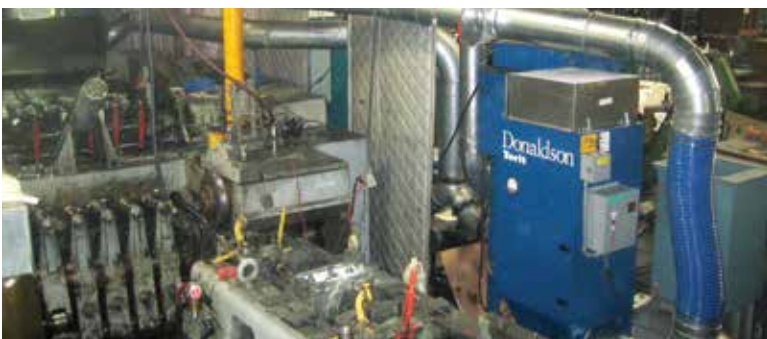
WSO on Cold Forming 1,200 cfm (2,038 m 3 /h)
