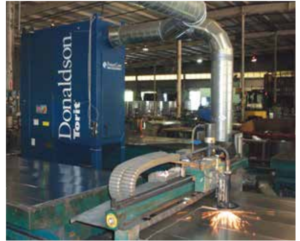
TG on Plasma Cutting 3,400 cfm (5,775 m 3 /h)
