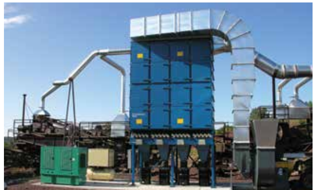
DLMC on Rock Crushing 41,000 cfm (69,645 m³/h)
