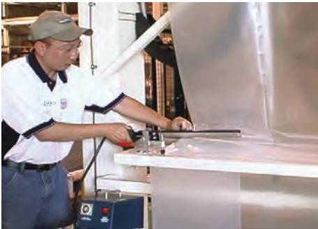
Splicing table with clamps folds down allowing fast and easy film roll splicing.
