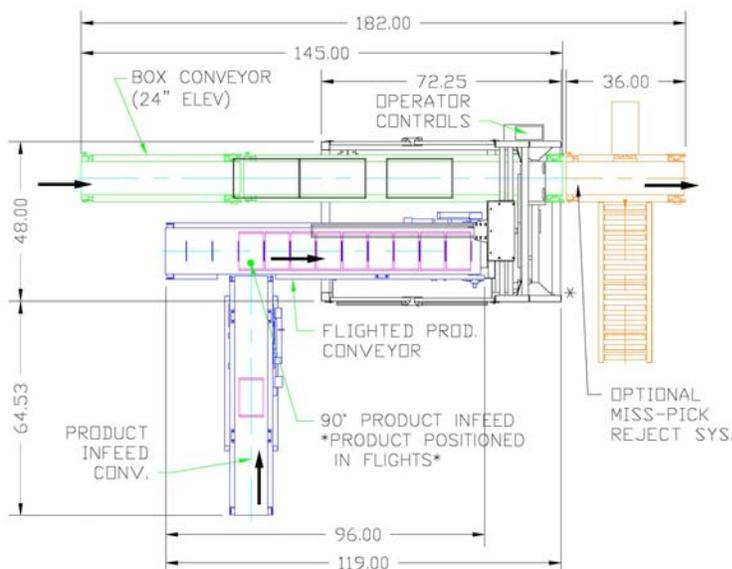
required package quantity has been indexed into position, the system’s pick head descends, securing the load by vacuum. The secured packages are lifted vertically and then placed within the staged case(s). This sequence is repeated until the case is fully loaded and then is discharged. When required, package rotation and overlapping is performed on the pick head itself.
