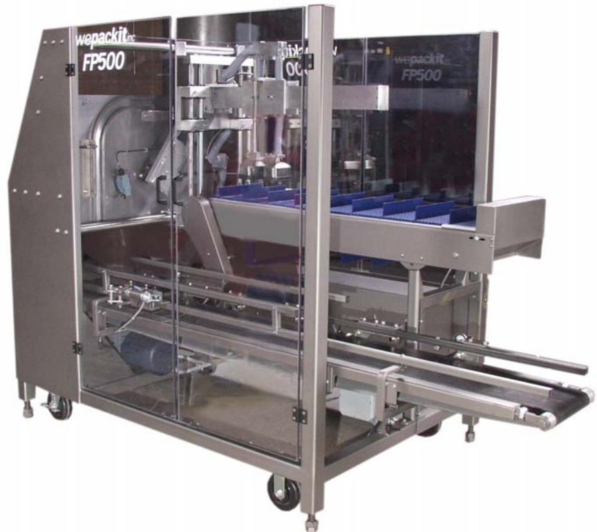
**SEQUENCE OF OPERATION** – Bags are “pretreated” to improve orientation, separation and center registration upon in-feed (if required). Introduced onto a registration controlling conveyor, packages are indexed forward until arriving into the system’s pick position. Formed and bottom sealed cases are in-fed and controlled in the staged pack position. Once the
