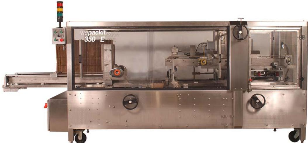
**Open Frame Design And No-Tool Handwheel Change Over** maintenance are greatly assisted by a standard open frame design, allowing full access to all erection sequences. Operating adjustment and magazine loading are positioned at standard operator height, providing for quick and easy access. Externally mounted **power-assisted** hand-wheels permit quick and effortless case size adjustment.
