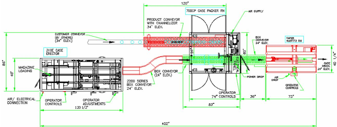
The **700CP** with a **320E** or **330E** gives a 25 case/min, robust construction capable of 24/7 harsh environments, and a smaller footprint.
