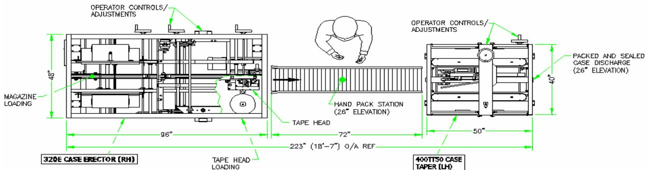
The live roller conveyor is divided into 3 sections: a live outfeed from the erector; a live infeed to the case sealer; and an operator foot controlled center section(packstation).
