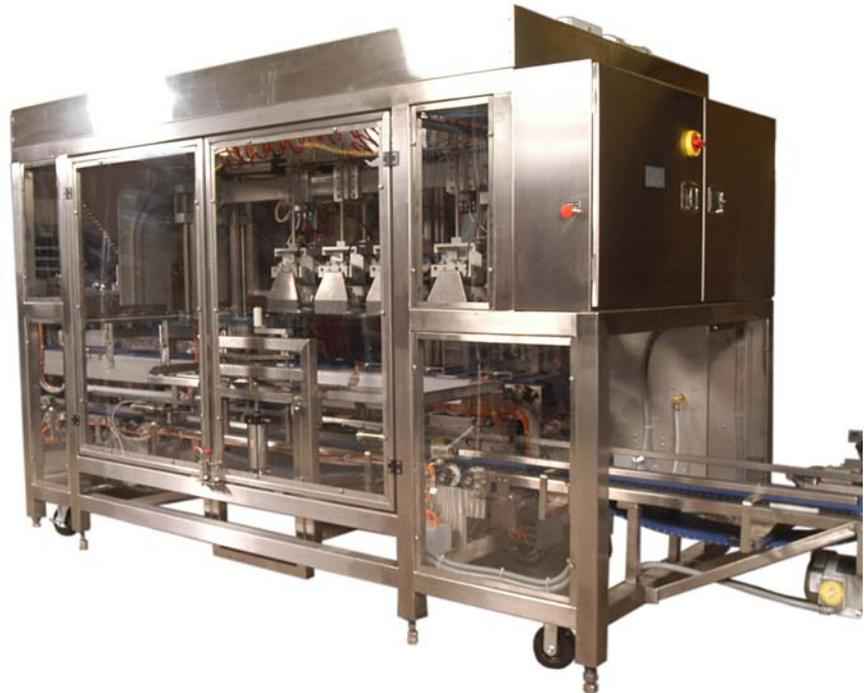
Once containers arrive into the pick area, the 350CP's heads descend on the product, securing it with vacuum or mechanical grippers. Containers are lifted vertically and placed within staged cases. As an on-demand system, the cycle is repeated until the cases are completely packed.
