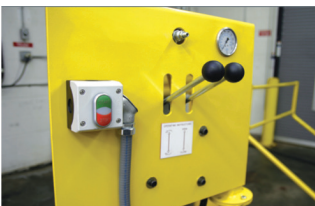
LEVERS: Basic control package will turn machine on/off, as well as clamp, un-clamp, and rotate
