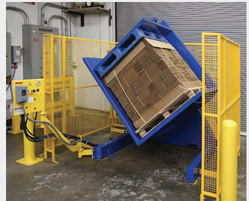
SAFELY TRANSFER CORRUGATE FROM A WOOD PALLET TO A PLASTIC PALLET
