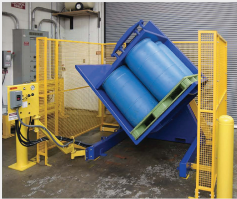
EASILY TRANSFER DRUMS FROM ONE PALLET TO ANOTHER
