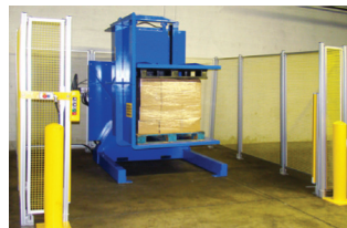
BOSCH GUARDING: Guarding which bolts directly to the floor with removable panels for maintenance access
