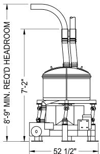
The Pfening Flow-Through Sifter sifts material while it is being pneumatically conveyed. Oversize material is deposited in a tailings container.
