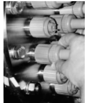
Screw the lamp socket cap into place
