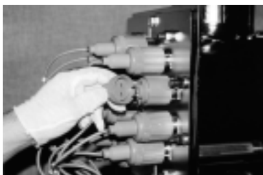
Firmly connect the lamp pins with the connector
