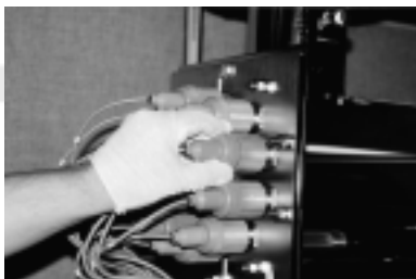
Screw the lamp socket cap on
