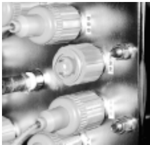
Lamp locked into compression nut
