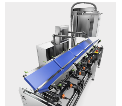
The V-shaped conveyor belt ensures gentle labeling of round or odd-shaped products
