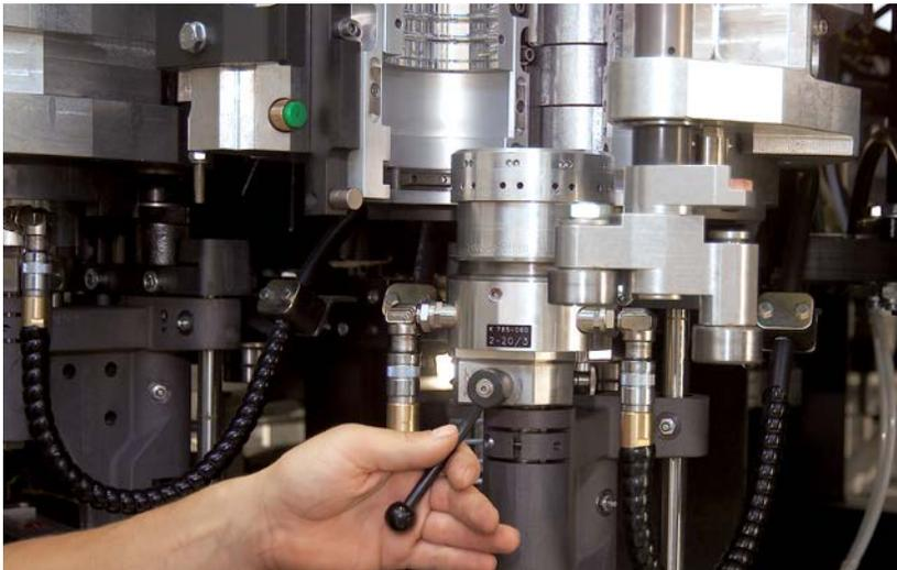
When it comes to change-overs, it is better to be quick. With the practical quick-change equipment, different preforms and bottles can be handled on the same Contiform without major time loss.
