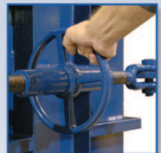
10-inch ratchet wheel is easier to operate than 6 or 8-inch wheels.
