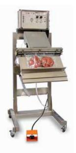
Seal length: 18" to 36", twin head: to 60" Seal width: 5/16"
