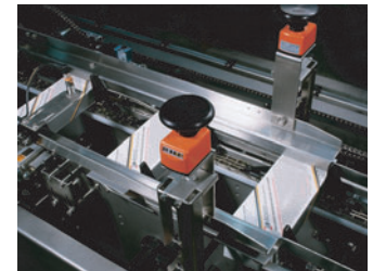
Optional digital readouts are used for consistent and faster carton size changeovers.
