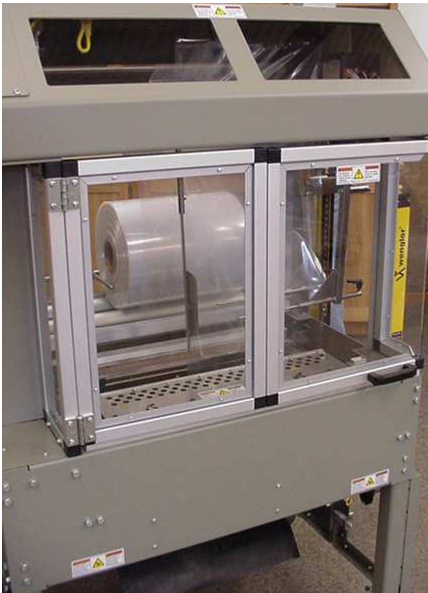
Figure 4-4 Hinged Safety Doors and Guards
