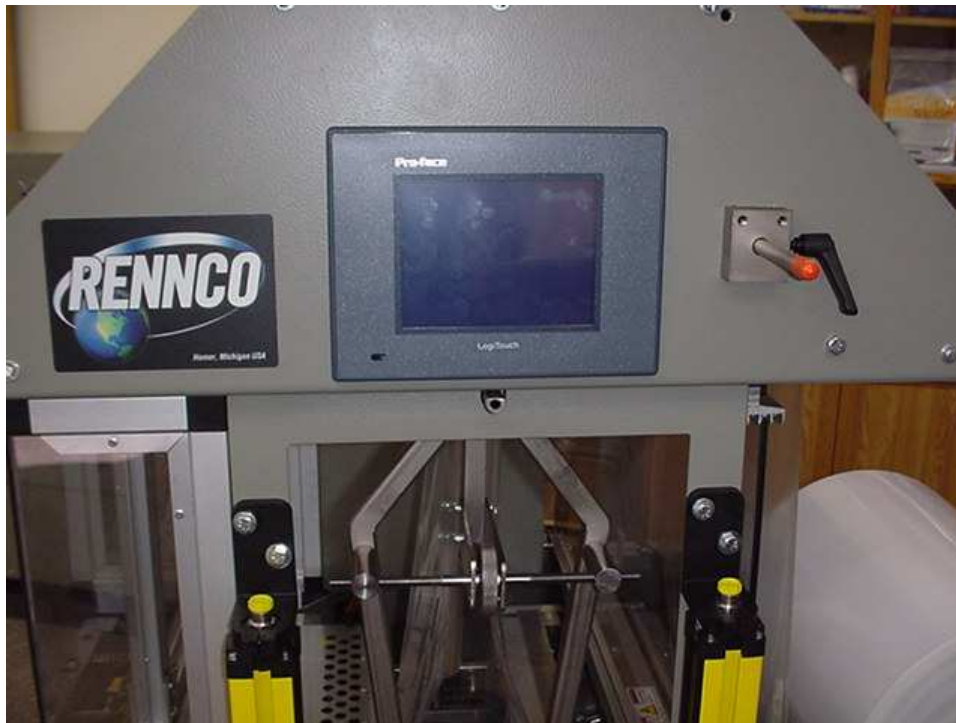
Figure 9-1 Operator Interface Enclosure
